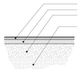
1.5" H.M.A. SURFACE COURSE IL-9.5, MIX "C" N50 2.5" H.M.A. BINDER COURSE, IL-19.0, N50 EXISTING AGGREGATE BASE COURSE. COMPACT AND PROOF ROLL EXISTING SUBGRADE
